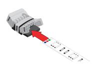
**1.** Peel back 1/2" of RGB Tape Light adhesive backing; insert end of RGB Tape Light section all the way into one side of connector.
