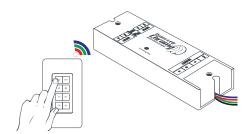
**4.** Turn on 120V AC to Power Supply and pair Receiver to Controller.
