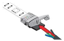
**2.** Leaving insulation intact, insert the 4 colored RGB wires into corresponding wire channel on long side of connector. Close cap and press gently with pliers to secure connection. The connector will cut through insulation to make contact.
