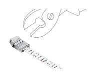
**2.** Close cap and press gently with pliers to secure connection.
