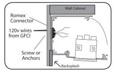
Secure APS – TR Series to wall with screws into each stud or use anchors provided. Strip wires and connect BLACK wire from romex to GOLD terminal and WHITE wire from romex to SILVER terminal. Ground all GREEN wires to PEM studs inside of back frame. When connecting two APS – TR Series, run Romex from piece A to piece B. Ground each section to the next.
