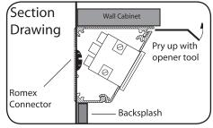
Turn power off at panel. Carefully pry open each piece with tool (provided). Insert Romex connector into hole. Pull wires into APS-TR Series.
