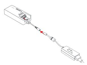
Insert the Male Barrel Connector on the Power Supply into the Female Plug Cable on the Receiver.
