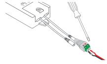
2. Insert Male Plug on Receiver into Female Barrel Connector. Use Flat blade screwdriver to loosen screws on Female Barrel Connector. Insert wires, Red wire to (+), Black wire to (-), and tighten screws.
