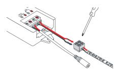
**5.** Use #1 Phillips to loosen the 4 terminal screws on 8MM-EZ Connector. Peel 1/2" of the adhesive protector from back of LED tape light, insert into connector, evenly tighten screws. Insert wires from Receiver into terminals, Red wire to (+) side of tape, Black wire to (-) side of tape; tighten screws.
