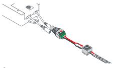
**3.** Use #1 Phillips to loosen the 4 terminal screws on 8MM-EZ Connector. Peel 1/2" of the adhesive protector from back of LED tape light, insert into connector, evenly tighten screws. Insert wires from Receiver into terminals, Red wire to (+) side of tape, Black wire to (-) side of tape; tighten screws.
