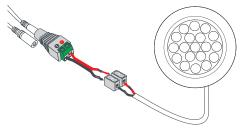
3. Cut Female Plug on Puck Light and insert wires, matching Red wire to Red, Black wire to Black into EZ-WSC Connector.
