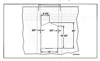
For AS-1075, mark the measurements, as shown, for the cut out onto the wall panel. Try to center the opening in the stud pocket. The wall stud opening shown is 16" on center, which creates a 14-1/2" opening.
