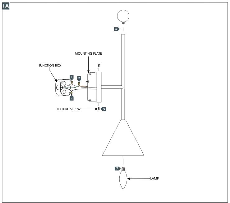
Secure the mounting plate to the junction box.
