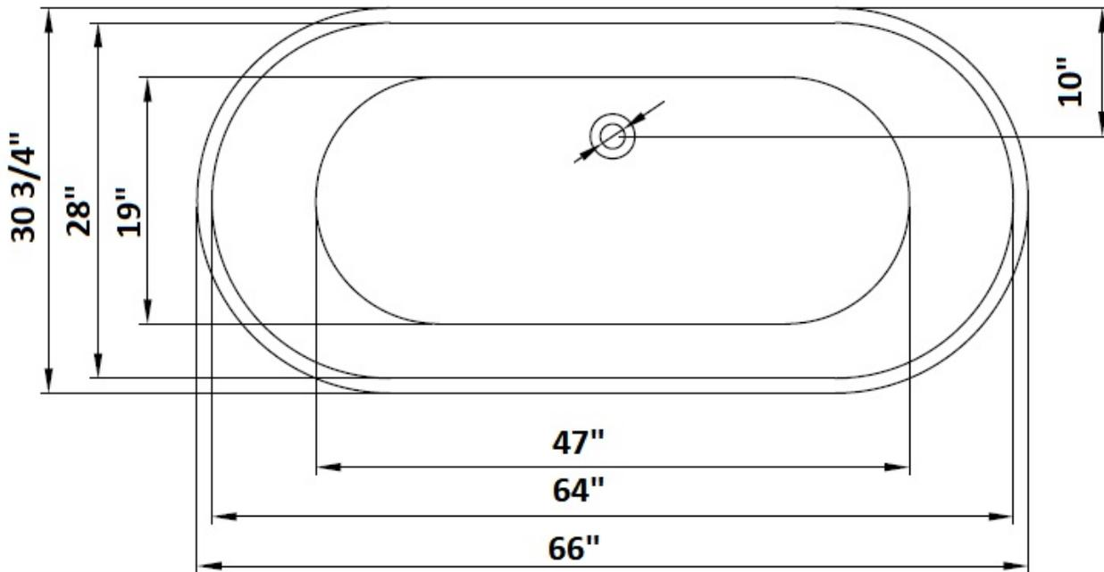
**The Overflow channel is molded into the interior tub wall. Drain is included.**
