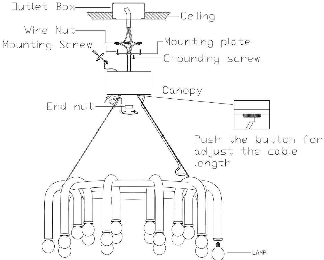
**WIRE NUT/TAPING DIAGRAM**
