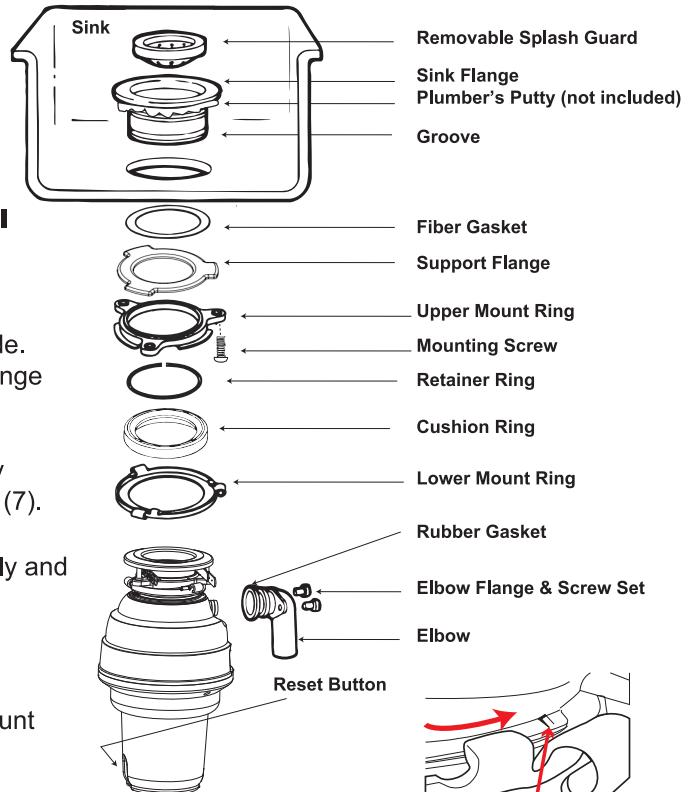
d. **Place a heavy object, such as the disposer (use a towel to prevent sink scratching) on top of the Sink Flange to hold it down.**
