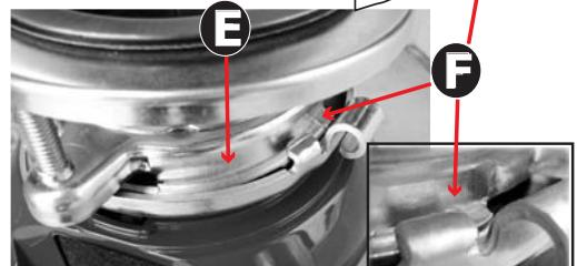
As the Lower Mount Ring is turned counter clockwise each tab slides up onto the Upper Mount Ring Ramp (E) and locks in position over the Ridges (F).
