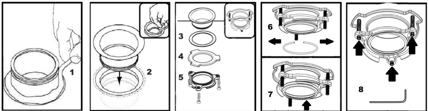
c. Be sure the sink is clean. Load the underside rim of the sink flange with plumber's putty (1). From top of the sink, push the sink flange down against the sink opening to make a good seal (2). DO NOT MOVE OR ROTATE the sink flange once it has been seated or the seal may be broken.
