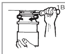
D. To remove remaining mount system from the sink, loosen mount screws, push mount ring up. Under it is the snap ring. Use screwdriver to pop off ring (see 1D). Remove mount ring, protector ring and gasket from sink flange. Some mounts will require the unscrewing of a large ring holding the sink flange in place. Pull sink flange up through sink and clean off old putty from sink.
