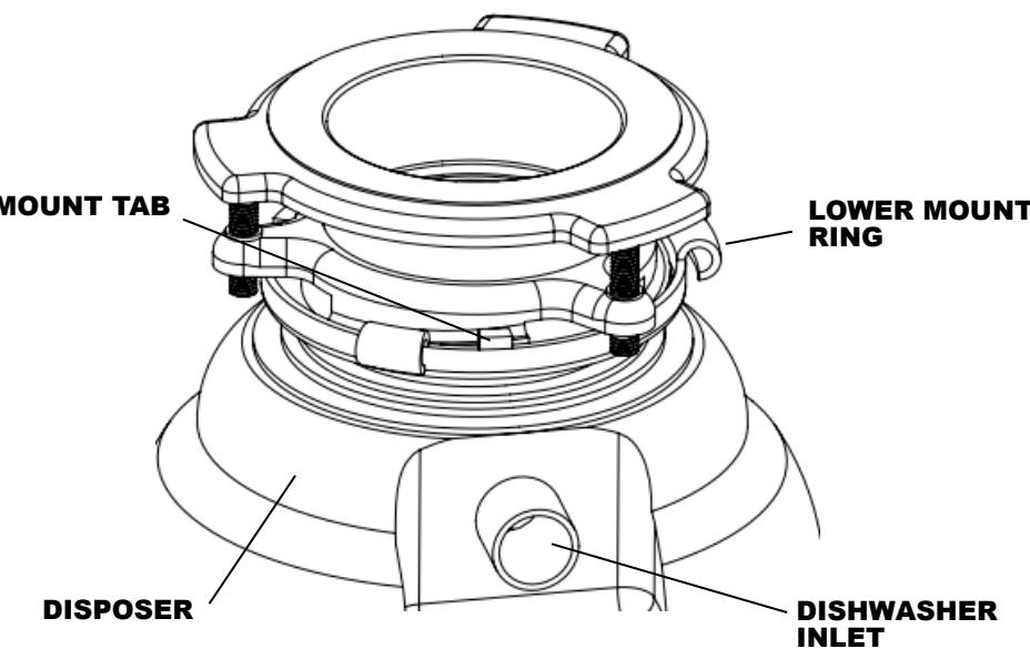
NOTE: Cushion Ring included between the Upper Mount Ring and Lower Mounting Ring.
