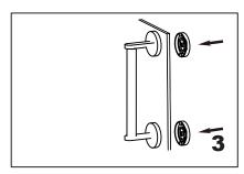
Add the end caps on the fixing brackets, make sure the set screws holes in the bottom.
