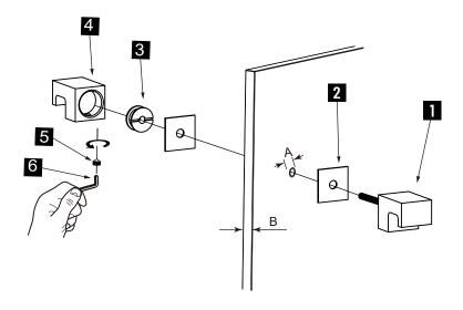
1.Knob-A x 1 2.Clear Gasket x 2 3.Fixing Bracket x 1 4.Knob-B x 1 5.Set Screw M5 x 1 6.Allen Key 2.5mm x 1
