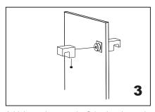
Add the end cap on the fixing bracket,make sure the set screw hole in the bottom.
