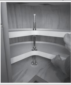
From the top slide one shelf, the other Shelf Support, and then the other shelf onto the Pole Assembly. Slide bottom of Pole Assembly into the Bottom Mounting Support.
