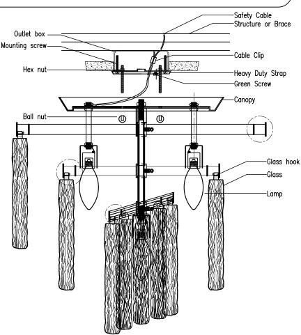
**3.** Fasten the ground wire to the green or bare copper wire in the outlet box or the green screw on the heavy duty strap.
